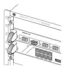
Figure 17: Installed XFP Module (Summit family switch and BlackDiamond 8800 series switch)
